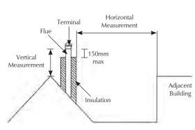
The vertical measurement is the lowest from either the point of discharge or 150mm above insulation.
